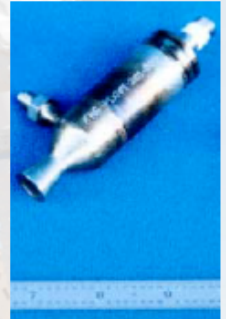
H2O2 Gas Generator
