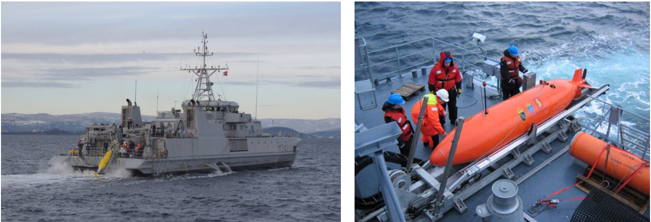
Figure 3: The RNoN minehunter KNM Karmøy with the HUGIN I (left), and HUGIN 1000 on the aft deck (right)
