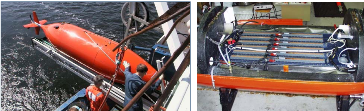
Figure 1: HUGIN 3000 with the battery compartment (right) showing the 50 kWh Al/HP semi fuel cell.
