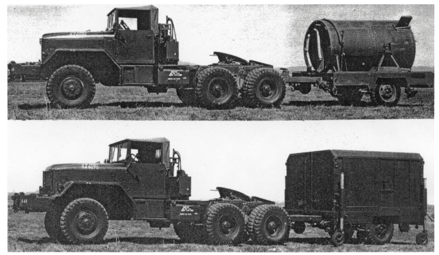
Figure 24. The aft unit is transported on the XM480 trailer. Like the other two trailers, the upper portion or cover of the trailer is removed by lowering a set of four extendable legs (shown in bottom photo). The cover is then elevated by a series of jacks and the entire assembly is pushed to the rear by battery personnel thereby uncovering the aft unit.
