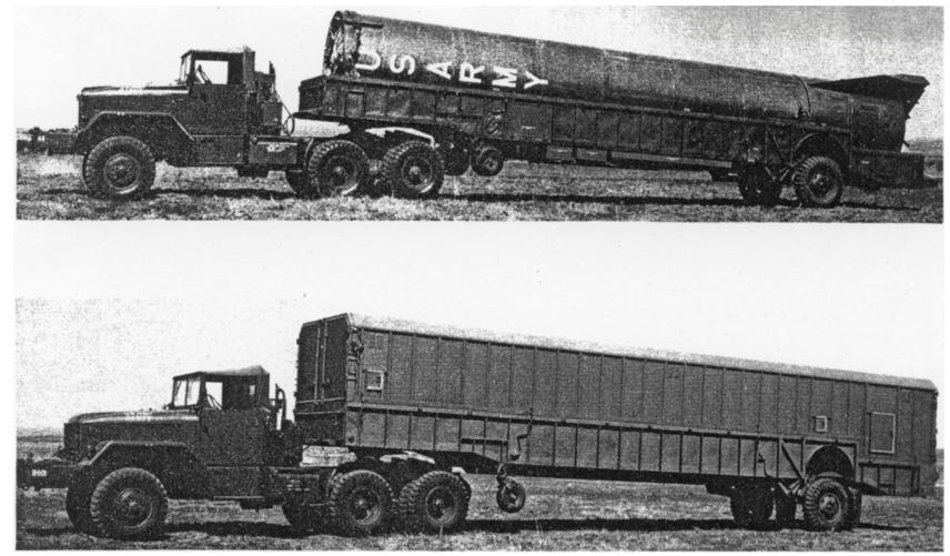
Figure 23.The missile is transported into the battery area as three separate units. The thrust unit is the<br/>largest of the three and is carried on the XM482 semitrailer. The cover (shown in bottom photo) is removed prior to
