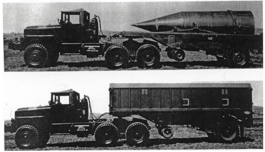
Figure 25. The warhead arrives in the battery area on the XM481 semitrailer. After the warhead and the aft unit have been uncovered, the aft unit is removed from its trailer by a standard 5-ton wrecker and is mated to the warhead. Once mated this portion of the missile is termed the "body." The bottom photo shows the trailer with the cover mounted.
