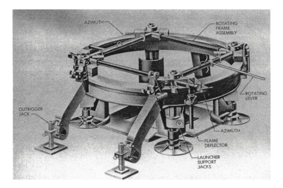
Figure 27. The XM74 launcher is used to orient the missile vertically and to aline the selected reference fin toward the target. The wheel and axle assembly is removed when the launcher is emplaced.
