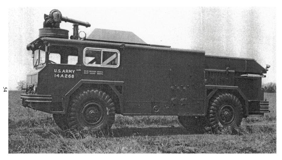
Figure 41. The fire truck carries 1,000 gallons of water and is used to neutralize spilled propellant or to extinguish small fires which may ignite when the missile is fired. The truck normally tows a four-wheeled water trailer which contains a 2,000-gallon reserve.
