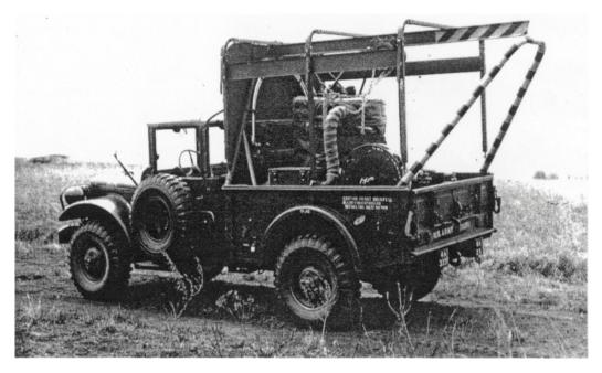
Figure 40. The XM387, hydrogen peroxide servicer, carries a 78-gallon drum of concentrated hydrogen peroxide which is used to generate steam to operate the missile's propulsion system. The propellent loading sequence is: alcohol, LOX and hydrogen peroxide.
