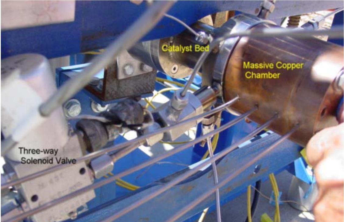
Figure 2. Details of Test Thruster
