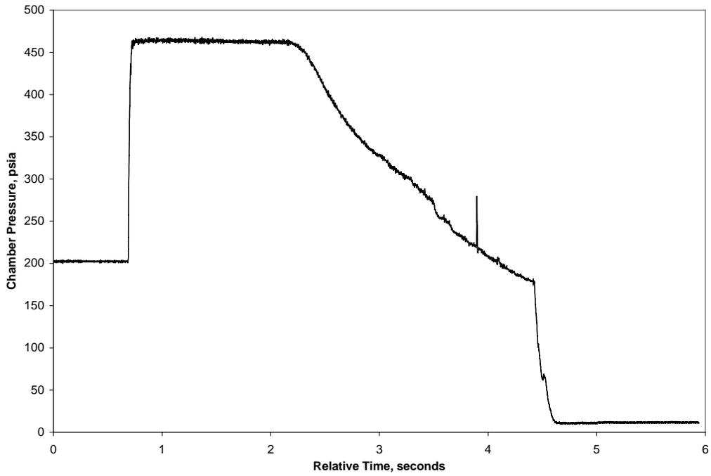
**Figure 7. Measured Chamber Pressure for Test 112103\_004**
