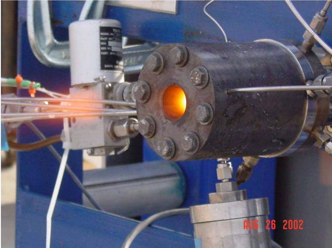
**Figure 9. Plume Photo of Test 082303\_007 During Bi-Propellant Operation**
