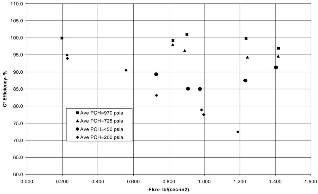
Figure 6. Flux Test C\* Efficiency Data Comparison
