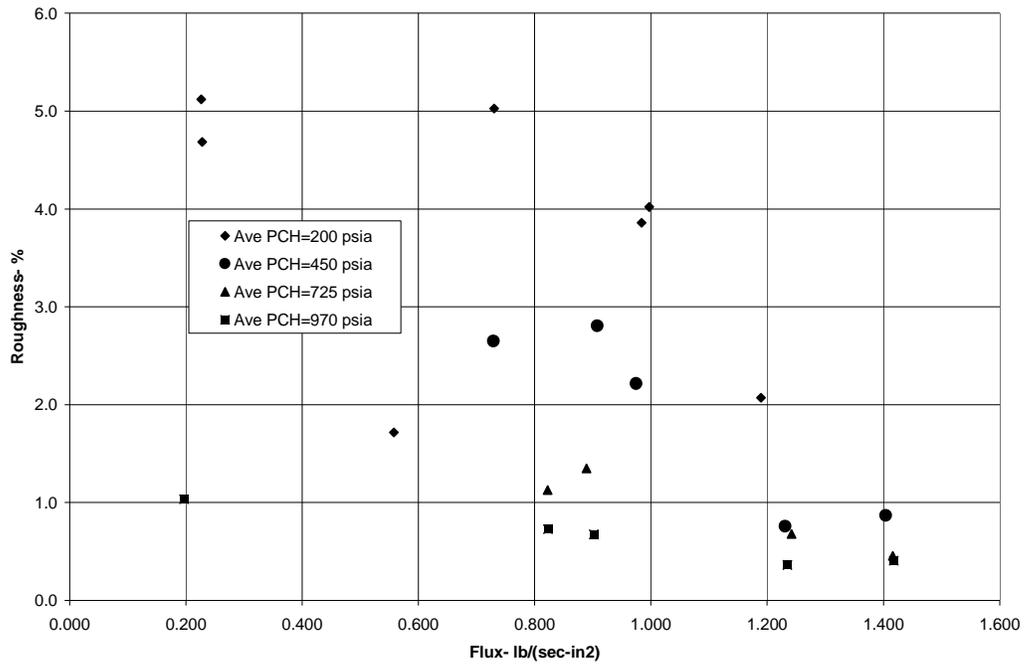
**Figure 5. Flux Test Roughness Data Comparison**
