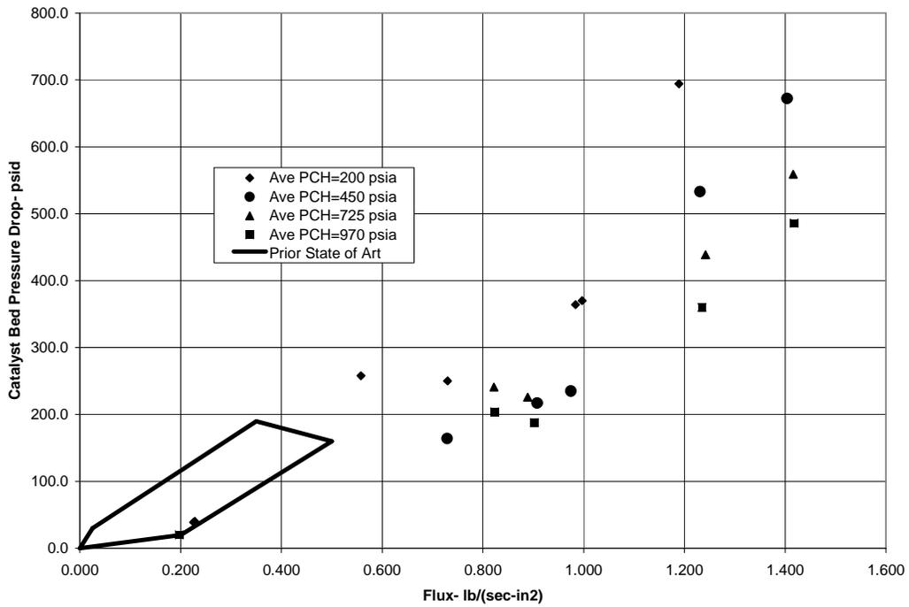
Figure 7. Flux Test Catalyst Bed Pressure Drop Comparison
