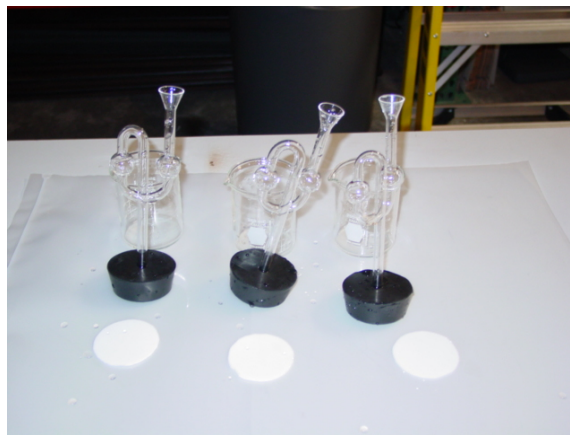
Figure 4 – Stoppers, Teflon Shield, and Water Trap Test Set-Up
