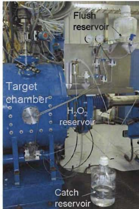
Figure 5. RLLS is shown as implemented on the LANL two-stage gas gun. The H_2O_2 reservoir and several valves are located on a plate situated so that the components are above the target cell inside the target chamber to facilitate a gravity feed to the cell. There is also a large container of water on the plate that allows flushing the system after an experiment.
